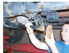
**Step 8: Install new Patented Forged Torsion Key and reposition back into proper position in the vehicle Crossmember and the anchor points at the front of the vehicle. Be sure Torsion Bar passes through Torsion Key by a minimum of 1/8" to 1/4"!! (Figure E)**
