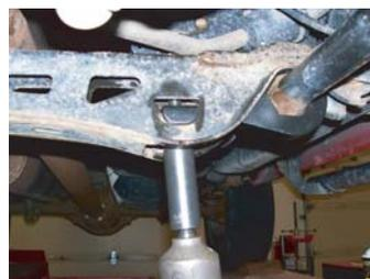
**IMPORTANT!: The SHOCK is the limiter of the amount of available lift, NOT the number of threads available on the Adjuster Bolt! Be sure adequate shock travel is evident after adjustment.**
