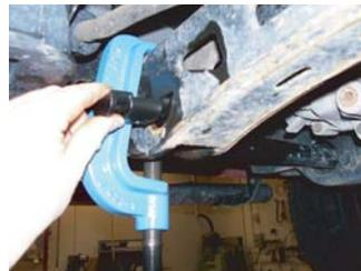
**Step 11: SLOWLY** release tension on the unloading tool until it can be fully removed.
