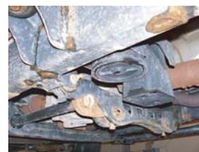
**Step 3: Locate the Torsion Keys.** They are found where the Torsion Bars are received into the Crossmember between the frame. **(Figure B)**
