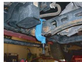
**Step 6: Remove the Threaded Adjuster Bracket, and SLOWLY release tension on the unloading tool until it can be fully removed.**
