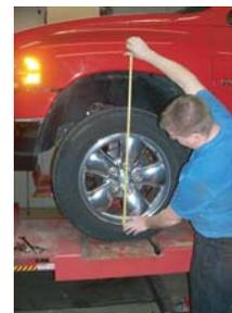
**Step 2: Position vehicle on a flat surface or automotive lift.** Suspend front wheels, lifting by the frame with a floor jack or lift jack. Secure using jack stands.
